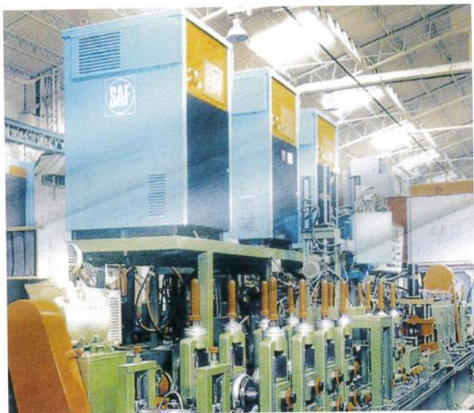
食品衛生及鍋爐熱交換器用製管機 Sanitary Tube(Food Industry) & Heat-Exchanger Tubes Welding Machine
